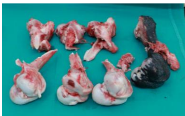
Fig. 5. Femur after dynamic testing at an impact velocity of 5 m/s
