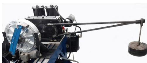
Fig. 6. Level system for applying the to flange of the specially designed coupling
