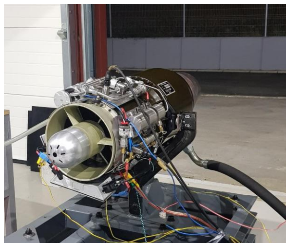
Fig. 7. Final version of the turbojet engine TJE-200 with subsystems at the test stand
