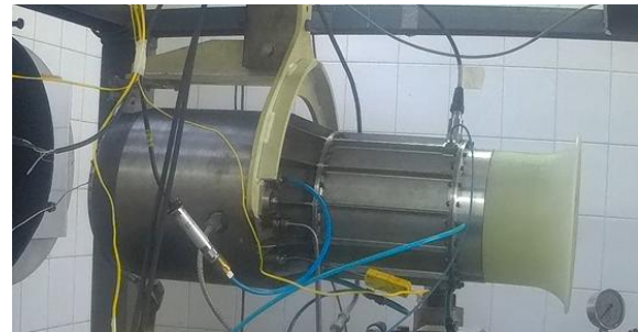
Fig. 3. TJE-200 at test without nozzle
