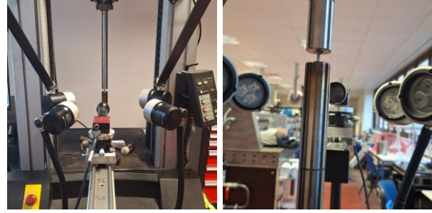
Fig.2. DIC arrangement with four continuous LED lights providing symmetric illumination of the gauge region – left; magnified - right
