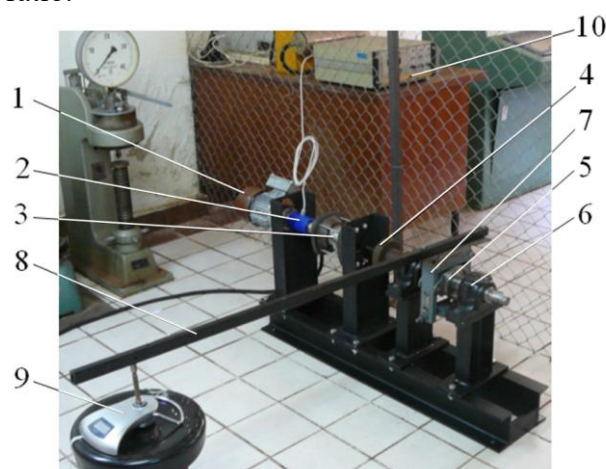
Fig. 2. Dynamic testing rig for planetary gear trains; 1 electric motor; 2 torsion meter; 3 planetary gear train; 4 gear coupling; 5 brake drum; 6 bearing; 7 friction brake; 8 lever; 9 force meter; 10 data acquisition system
