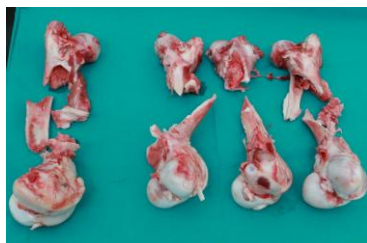
Fig. 6. Femur after dynamic testing at an impact velocity of 10 m/s
