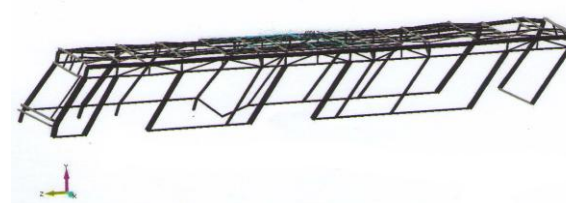
Fig. 3. Bus model in the deformed state (first loading case).
