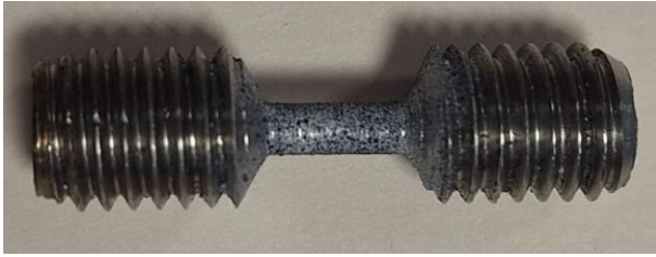
Fig. 1. Threaded tensile specimen (S1100QL) with DIC speckle applied to the gauge.
