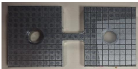
Fig. 1. Flat dog-bone tensile specimen with central neck prepared for testing; DIC grid applied over the gauge region
