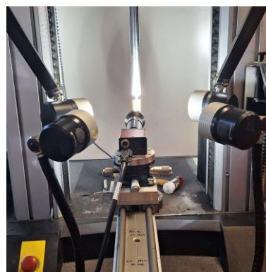
Fig. 2. DIC arrangement with four continuous LED lights providing symmetric illumination of the gauge region
