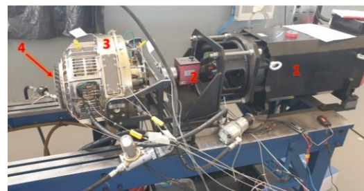
Fig. 7. Test stand with high speed gearbox for airplane application: (1) drive electromotor, (2) torque meter, (3) propeller gearbox, (4) free turbine
