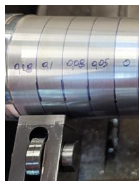
Fig. 1. Surface of Al6088 workpiece with cylindrical sections treated by ball burnishing under different feed rates
