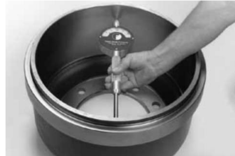
Fig. 3. Measurement of drum deformations.
