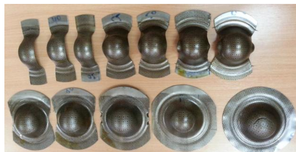
Fig. 1. Sheet metal samples made of DC04 material for FLD determination
