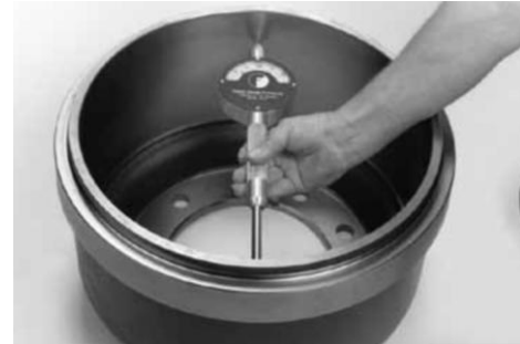
Fig. 3. Measurement of drum deformations.
