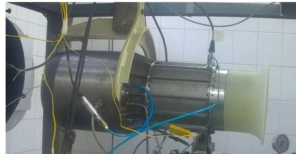
Fig. 3. TJE-200 at test without nozzle
