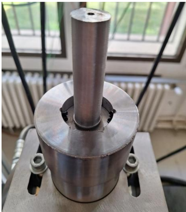
Fig. 4. Assembly of the joint and auxiliary components on the pulsator after the first test series.
