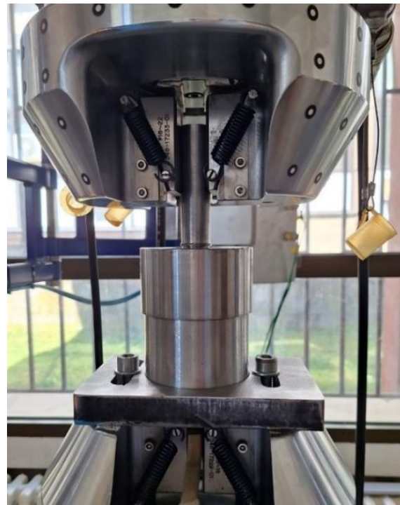
Fig. 3. Assembly of the joint and auxiliary components on the pulsator.
